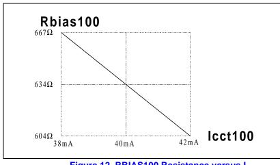
Figure 12. RBIAS100 Resistance versus I<sub>CCT100</sub>
